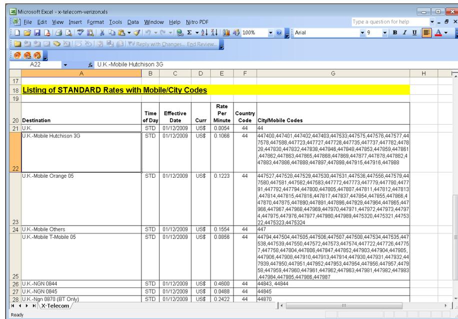
You can easily process such files – you just need to specify which character (e.g., comma (,), semicolon (;) or something else) will be used to separate the individual prefixes in the **Delimiter For Multiple Destinations** field. This way, during the upload, the system will treat each occurrence as if there is a separate row in the table for each prefix.
