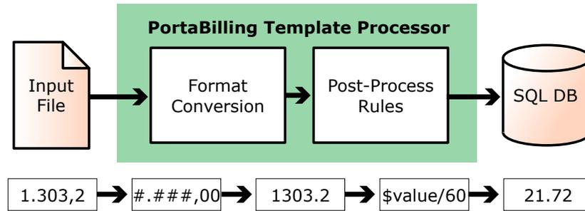
Such a template (called an upload template) is defined via a user-friendly rate upload wizard during the first upload of rates from a tariff with a specific format.
