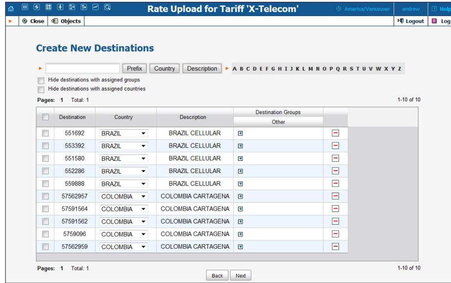
Carriers frequently send rate files containing prefixes that have not yet been defined in your system. These prefixes must be added into the system in order for rates to be created for them – so the big questions are: ‘how will this affect the routing and billing on your system in general?’ and ‘how will other carriers and customers be affected?’
