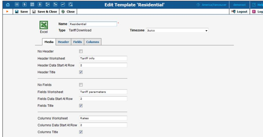
Here is a sample data file that matches this template. Note that “...Data start at row” means the first row with actual data, not including the title. For example, line 7 contains titles for column data, and so 8, the number of the first row with rate data (4066667...), appears in **Column Data Start At Row**.
