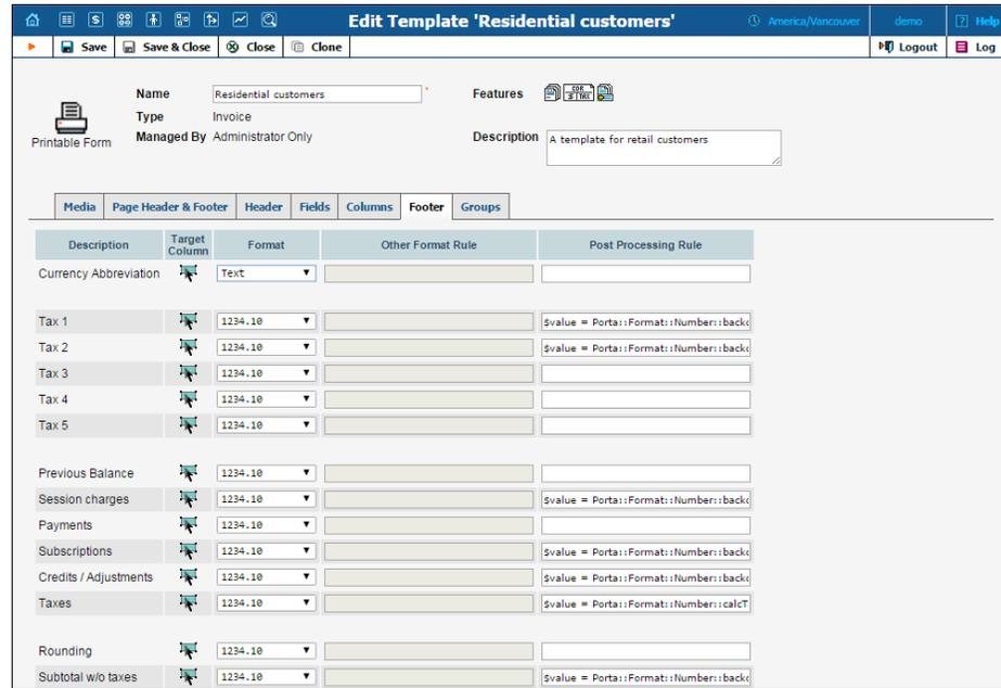
The PortaBilling® template library has a function which can be used to easily calculate the amount of certain types of tax. The `Porta::Format::Number::backcalcTax` function consists of three parameters:
